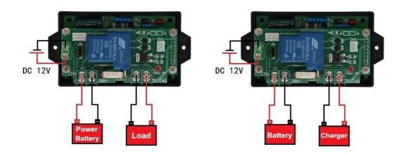
The wiring method on the left is applicable to the discharge measurement of the battery and the measurement of the DC circuit; the wiring method on the right is only applicable to the charge measurement of the battery. 2.2, wiring diagram of VAT1050, VAT1100, VAT1200, VAT1300 measuring voltage is 10-100V:
